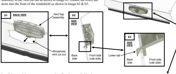
2. Install the remaining vent components (Item B) using supplied hardware as shown below in image b4 & b5.
