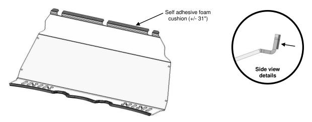
c) Find a clean flat area where you can safely lay down the windshield. Partially remove the protective film on both sides and install the vent grills (Item B &C) using supplied hardware (Item G) as shown.
