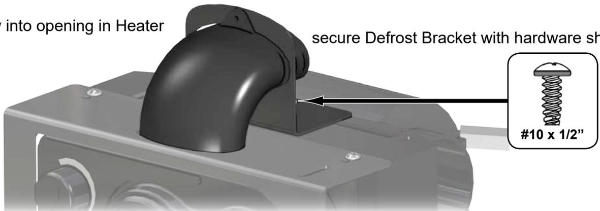
cut Duct to 32-1/4" and install to Elbow and secure with wire-tie
