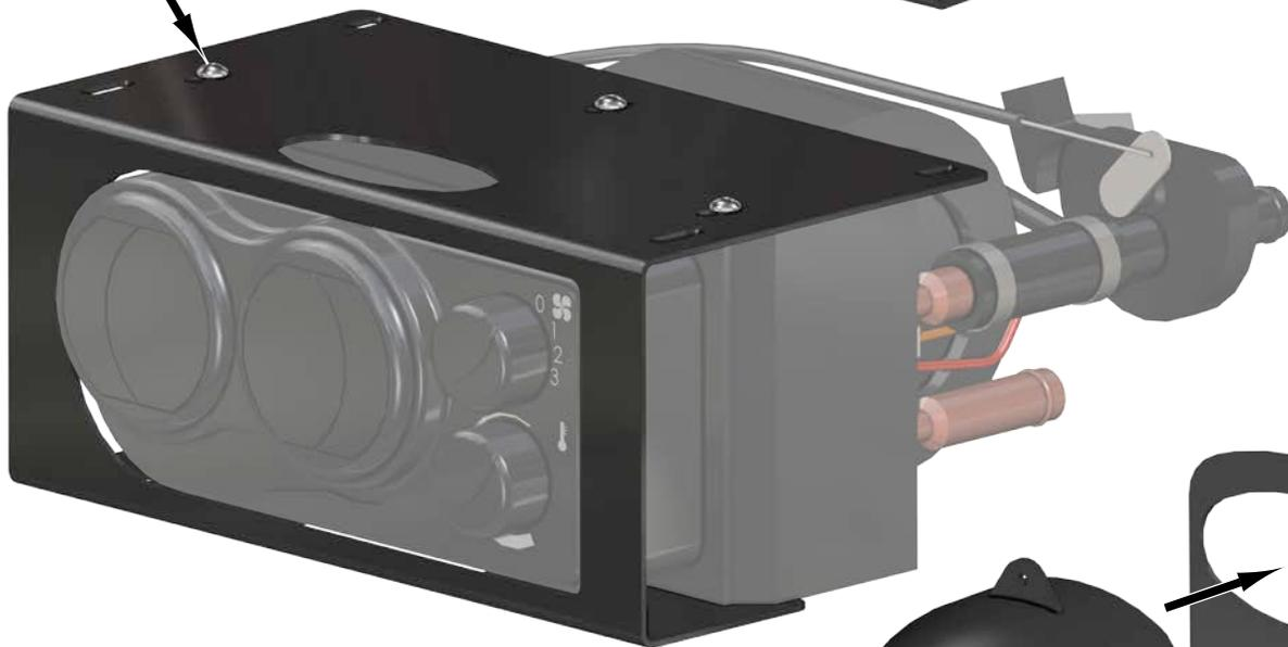
insert Elbow into Defrost Bracket
